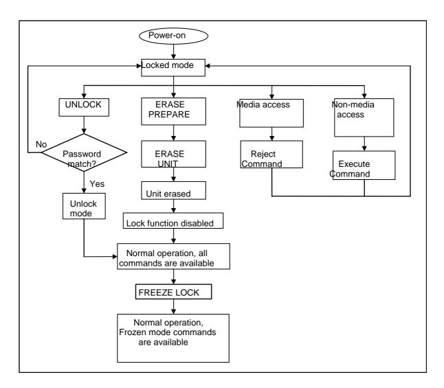
Figure 5 Password set security mode power-on flow
